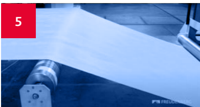
5 The filament web is then created.
