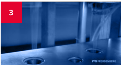
3 The melted blend is then spun to create endless bi-component filaments.
