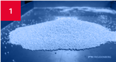
1 Polyester and polyamide chips ready for processing.
