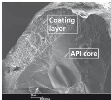
Figure 2: Exemplary scanning electron microscope image of a coated API particle.
