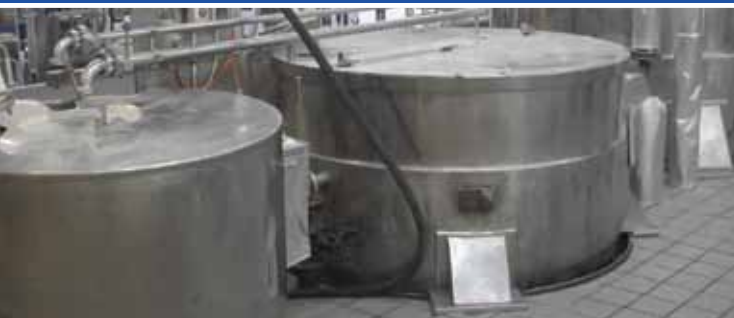
Mixing tank with two side tanks EMPL , year 1998, capacity 6000 ltr.
