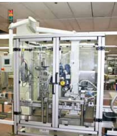
L6: cap sorting machine with mounting device (2 formats)
