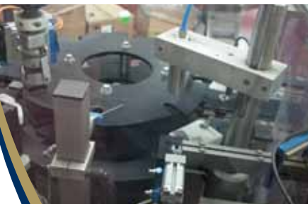
L6: cap sorting machine with mounting device (2 formats)
