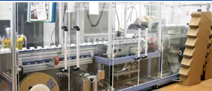
L57: horiz. Sleeve-wrapping machine LogicPak LPK Type 150 , year 2002, capacity 120 pieces per minute, format size 40-200 mm
