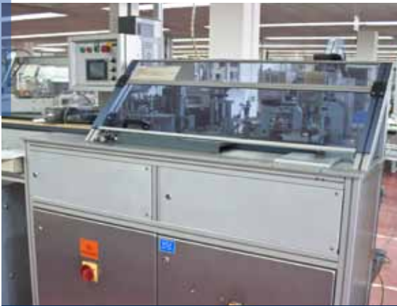
L32: Lauer PCS 085 control with feeding and completing unit
