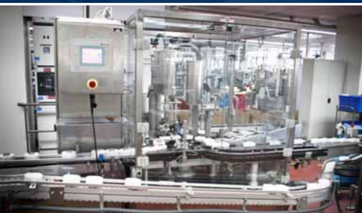
L47: caps inserting machine KUGLER type Flexocap (multiple formats available)
