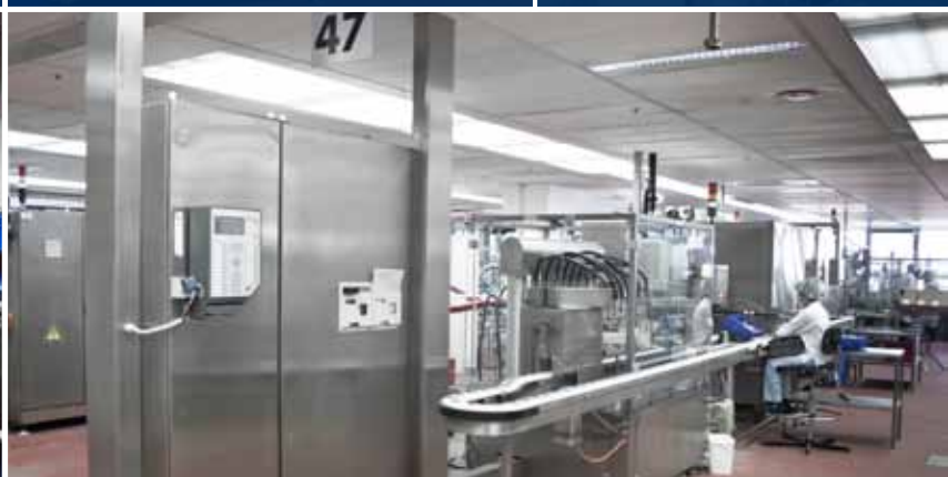
L47: Hotfilling system, year 2008, output of 60 pieces per minute
