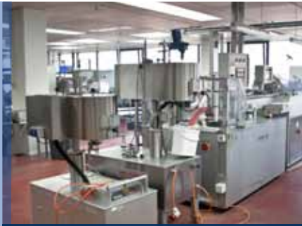
L32: Lipstick filling and packaging line WECKERLE SL 180, year 1994
