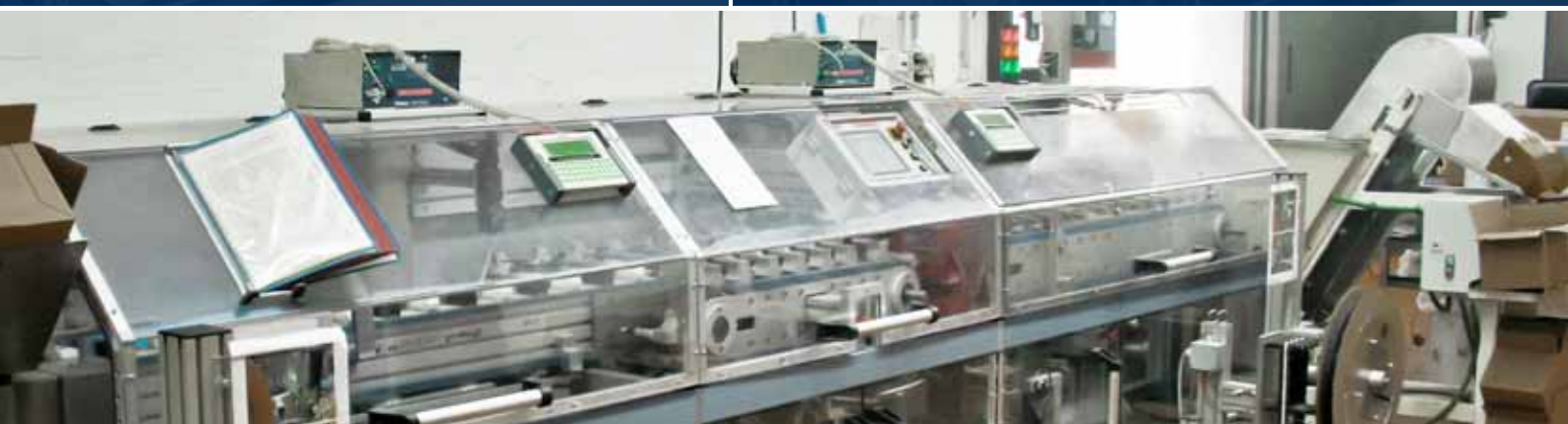
L59: horiz. Sleeve-wrapping machine double head-LPK LOGCIPAK Type 150 , year 2002, capacity 240 pieces per minute, format size 40-200 mm
