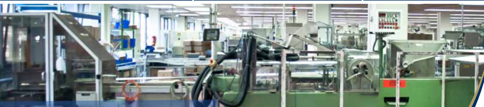
L44: retrofitted with laser marker MARKEM type SmartLaser 110 , year 2003
