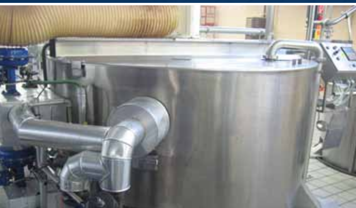
Mixing tank with two side tanks EMPL , built 1998, capacity 6000 ltr., Electr. agitator
