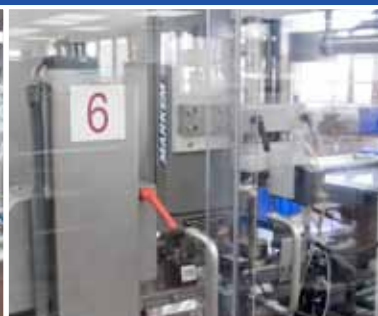
L47: Marking Systems MARKEN type SmartLaser 1102
