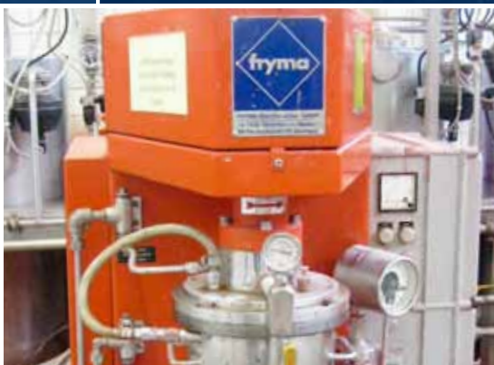
BALL MILL FRYMA type MS18, year 1986 with pigment-grinder (PVC balls)
