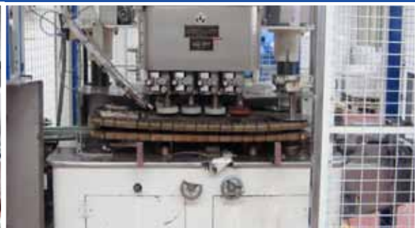
L7: cap mounting machine RESIN (4 - fold screw unit)
