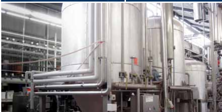
CIP CLEANING SYSTEM EMPL , year 1988, operating temperature 80 ° C - Detergents: Cleaning oil for boiler cleaning
