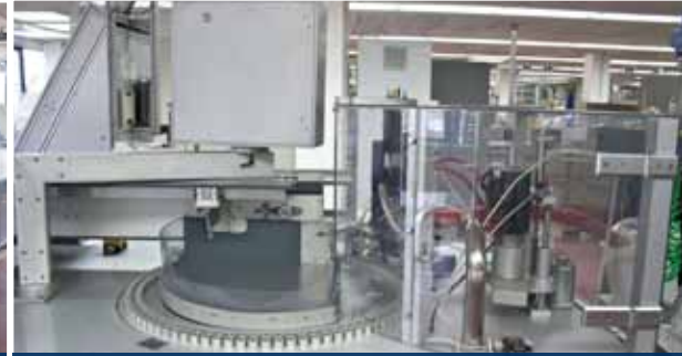
L32: rotary table with 180 molds (80-90° C)
