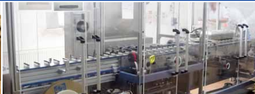
L58: horiz. Sleeve-wrapping machine LogicPak LPK Type 150 , year 2002, capacity 120 pieces per minute, format size 40-200 mm
