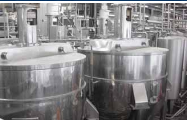
Mixing tank heatable (boiler SWEP)
