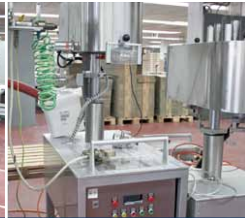
L32: double melting container with WECKERLE agitator
