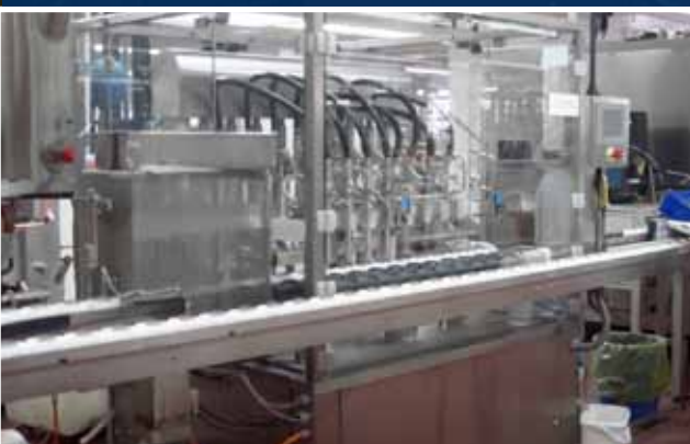
L47: 2x4 in-line filling-machine KUGLER type Linofill , max 90° C
