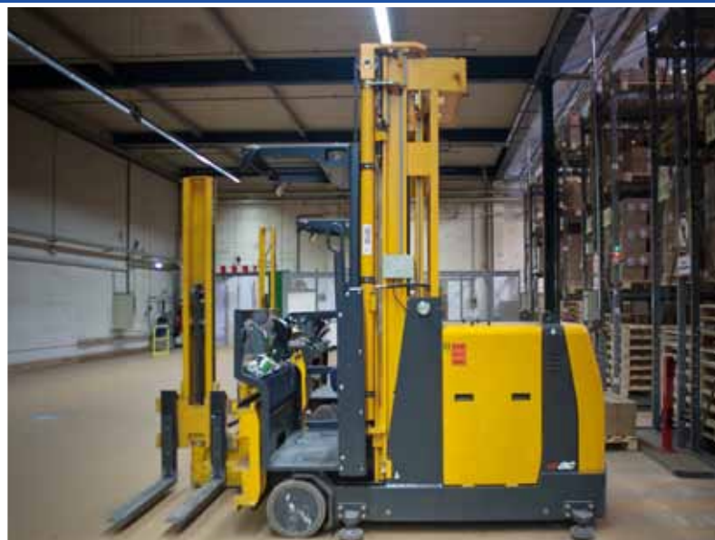
VNA trucks, narrow aisle forklifts e.g. Jungheinrich ETX-K125SG, year 1999
