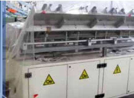
L24: Flat bag-sleeve packaging machine ILA-PACK type Carrera 1000PC, year 2000, product length 50 to 500 mm, width 20 to 230 mm
