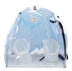
The CHE (controlled humidity environment) allows tablets to be made and tested under a specified humidity.
