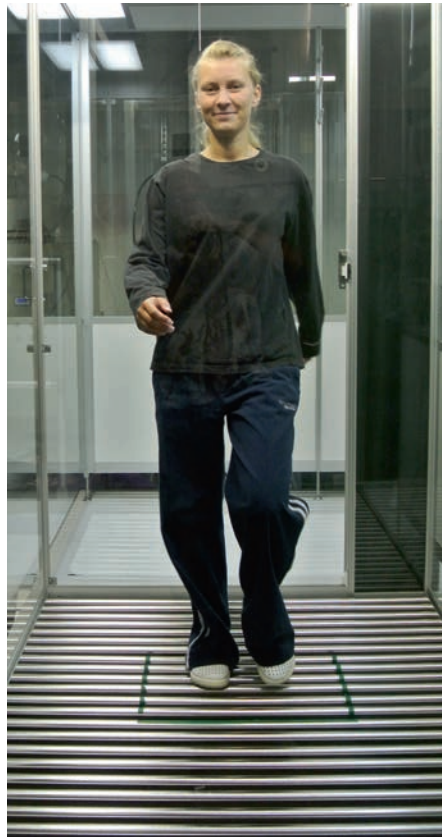
Here the tests being run are (left) on a person walking slowly while wearing 'street' clothes and (right) standing while wearing a cleanroom gown and bouffant cap
