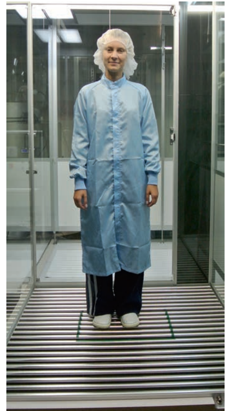
Here the tests being run are (left) on a person walking slowly while wearing 'street' clothes and (right) standing while wearing a cleanroom gown and bouffant cap
