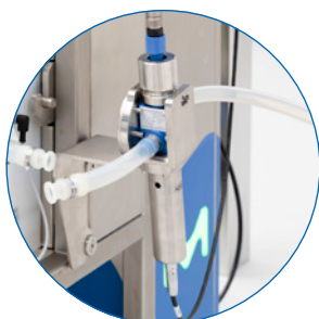
Pre-column instrumentation for conductivity and pH measurement
