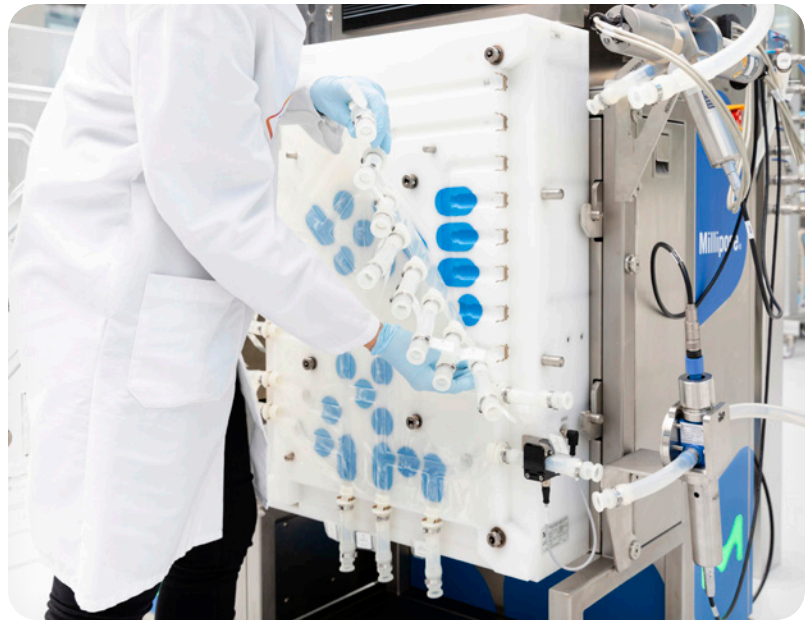
Mobius® Chrom 20 system clamshell and Flexware® clamshell assembly
